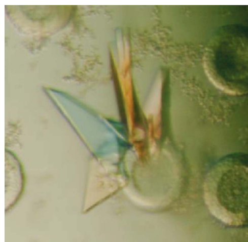
Figure 2 Crystals of (BACCR)NAT3 grown by the hanging-drop vapour-diffusion method in 1.37 M sodium citrate pH 6.5, 0.28 M NDSB-221 at 291 K. Crystal dimensions are approximately 100 × 100 × 50 µm.
